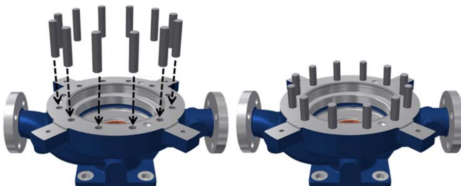
Figure 8.33 Inserting the continuous studs into the volute casing.
