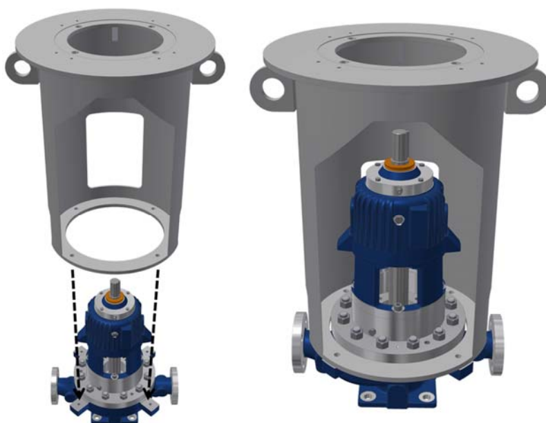
Figure 8.39 Placing the motor stool support over the volute casing. 图8.39将电机座支架放在螺旋壳上。
