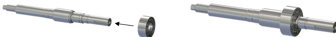
Figure 8.1 Placing the thrust bearings into the shaft. 图8.1将推力轴承装上轴。
