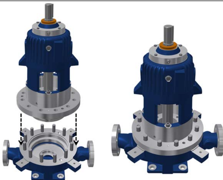
Figure 8.35 Placing the bearing bracket assembly into the volute casing.
