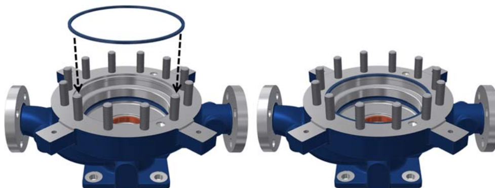
Figure 8.34 Placing the joint ring in the volute casing.
