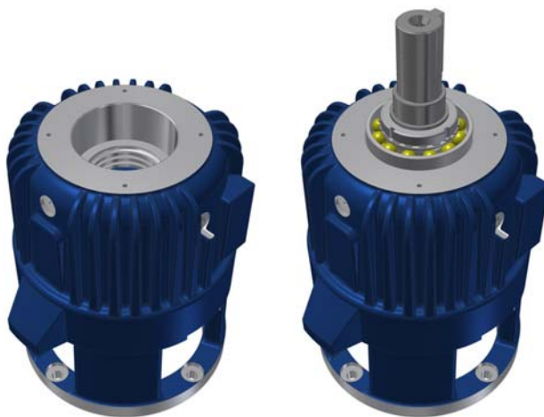
Figure 8.10 Placing of the shaft assembly into the bearing bracket.
