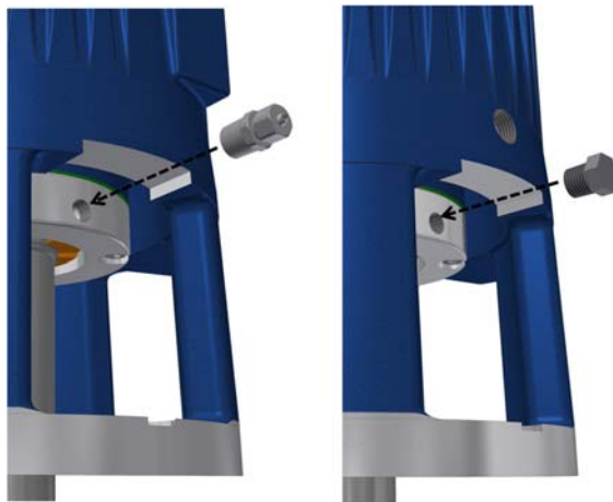
Figure 8.16 Inserting the grease fitting and the hex plug on the radial side.
