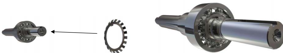
Figure 8.2 Positioning the lock washer into the shaft. 图8.2将锁紧垫圈定位到轴中。
