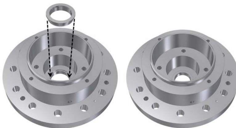
Figure 8.24 Positioning the throat bushing in the casing cover.
