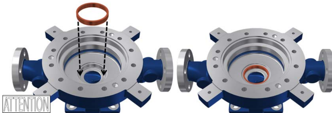
Figure 8.25 Placing the casing wear ring in the volute casing.
