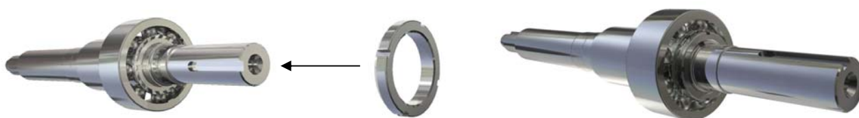
Figure 8.3 Placing the locknut into the shaft.
