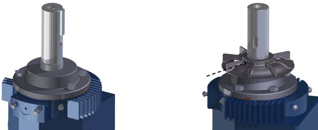
Figure 8.37 Placing the ventilator fan into the pump shaft.
